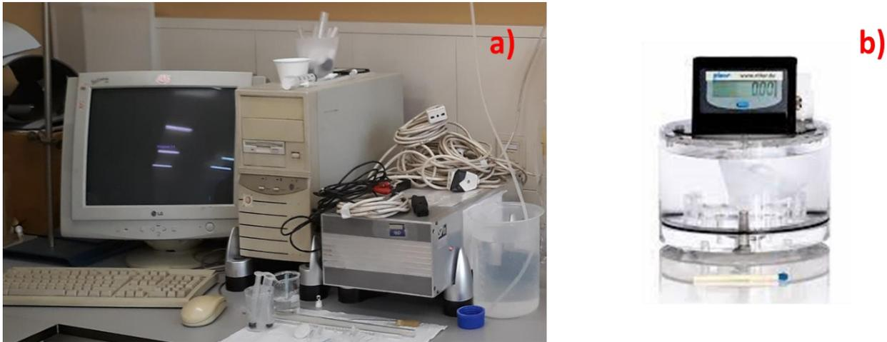
Figure 1 Picture of the (a) interface and (b) biogas measurement device connected to the lab-scale UASB system implemented at IRSA-CNR.
